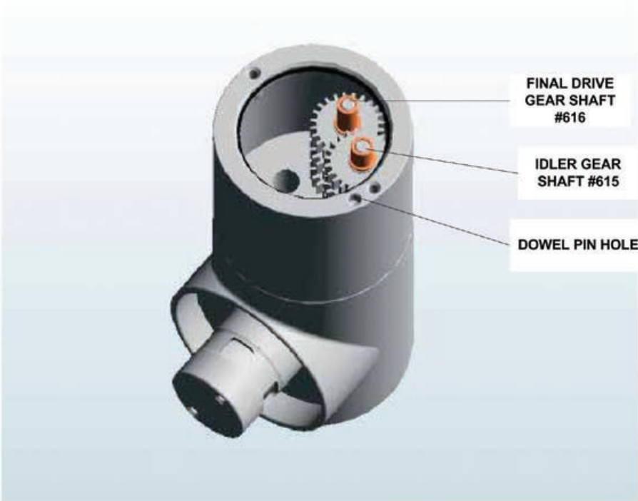
Photo 8 SEATING GEAR SHAFTS
